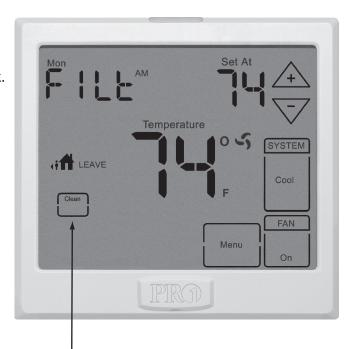
Hold down for 3 seconds, to reset filter reminder.
